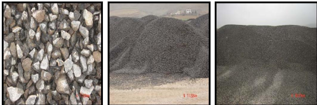
**Fig. 2.** Elazığ province basalt aggregates in the stone pit, (a) coarse aggregate, (b) medium aggregate, (c) fine aggregate [13]
