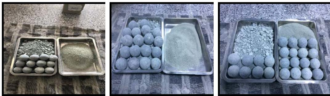
**Fig. 5.** Oversize – undersize remaining amounts of abraded basalt aggregates, (a) 12 balls, (b) 18 balls, (c) 24 balls
