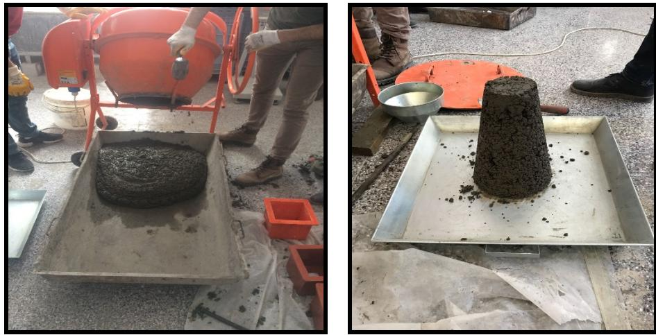
**Fig. 3.** Pouring of concrete and determining the fresh concrete properties of the mixtures: (a) Concrete mixer; (b) Slump test
