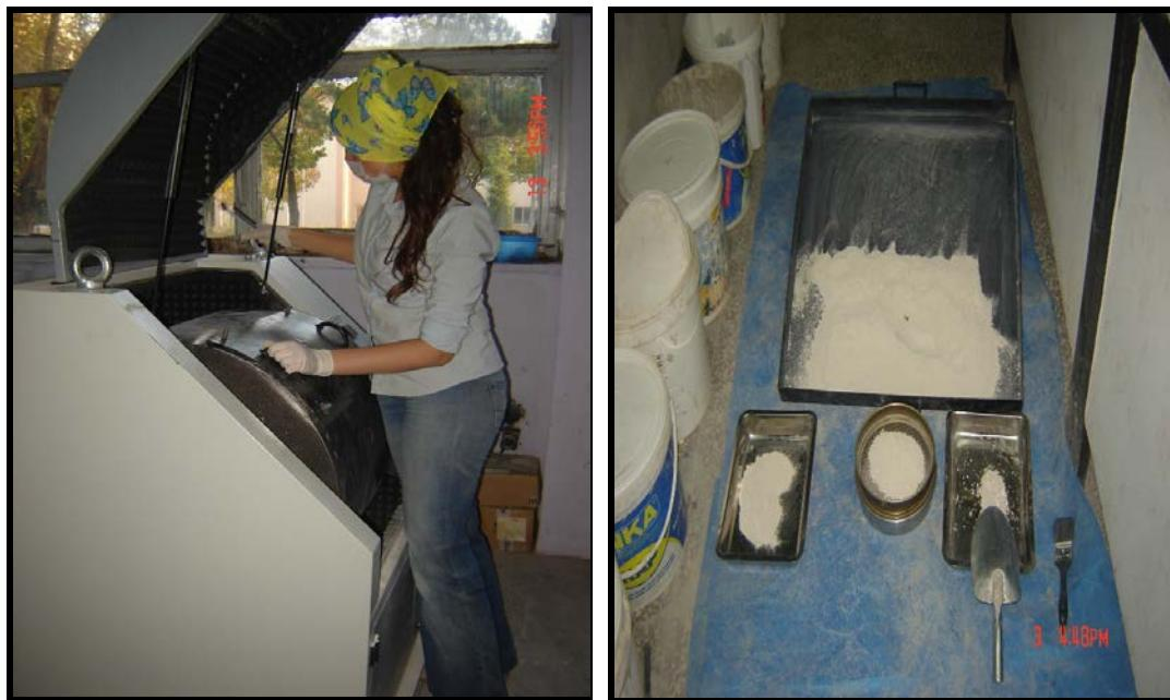
**Fig. 4.** Los Angeles abrasion device, (a) closing drum before abrasion, (b) after abrasion
